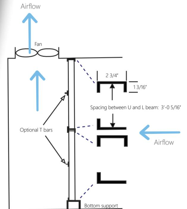
Andreae Filters are held in place by an inverted U-beam on top and an L-beam on bottom. If the booth has several rows of filters, each row is installed on top of the adjoining beam.
