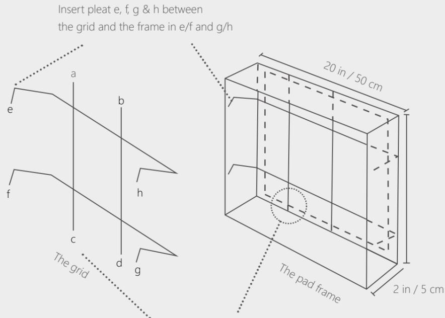
Tines a,b,c & d go behind the back of the frame to secure wire support while removing loaded filter
