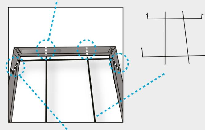
Wire support grid into filter frame
