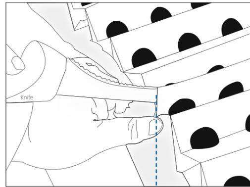
You will cut through two paper layers (plus synthetic material in the High range). Pinch the pleats on either side beneath the knife for additional control while cutting.
