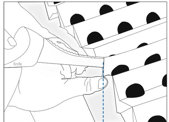
You will cut through two paper layers (plus synthetic material in the High range). Pinch the pleats on either side beneath the knife for additional control while cutting.
